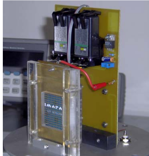
The detector array mounted on the AFEE board
