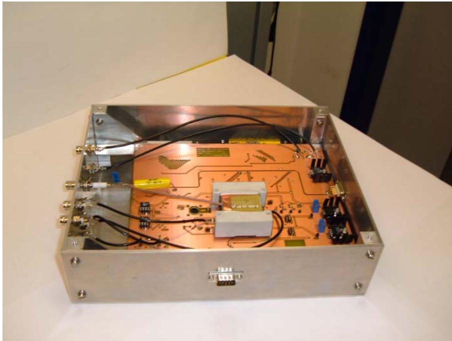
Prototype IMARAD 16x16 pixels equipped with 2 ASICs IDEAS XAIM 3.3
